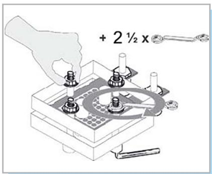
7. Tighten the nuts alternately a little at a time (max. two and one-half turns) until a gap of 4mm is left between the acrylic plates.
