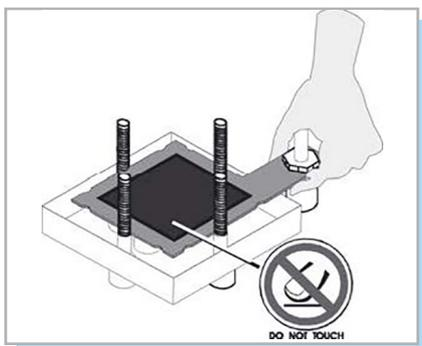
2. Place the positive (red) perforated plate on the acrylic housing. The thicker side of the seal, with the front of the banana jack, should face the acrylic. The electrode should point upward.
