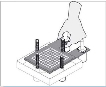
3. Holding the membrane electrode assembly (MEA) at two opposite corners, place it upon the perforated plate.
