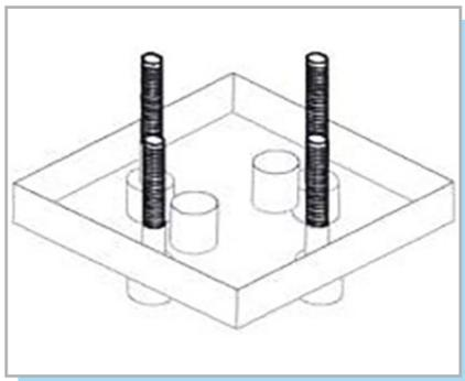
1. Place a washer over each of the four bolts. Insert the bolts into one of the housing plate and turn it upside down so it is resting on the head of the bolts.
