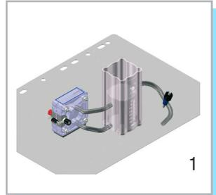
2 . Connect the electrolysis side of the gas storage tank to the connections on the hydrogen side of the electrolyzer with two short tubes. The gas storage tank serves as a hydrogen storage tank.
