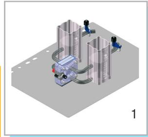
2 . Connect the upper and lower connections of the electrolyzer to the corresponding connections on the electrolysis side of the gas storage tanks with four short tubes.
