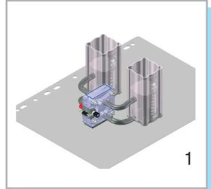
2 . Connect the upper and lower connections of the electrolyzer to the corresponding connections on the electrolysis side of the gas storage tanks with four short tubes (fig. 1).
