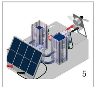
2 . When the gas storage tanks are filled, excess gas escapes as bubbles. Hydrogen production has to be stopped.
