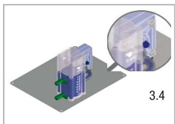
**NOTE:** The rising water level can easily be seen inside the cell. If air bubbles form they may interfere with the system. Allow the process to run until you see no more air bubbles.
