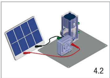
3. Oxygen is produced on the positive side of the cell, and hydrogen on the negative side. As the cell is operated in fuel cell mode with atmospheric oxygen, only the hydrogen will be collected in the gas storage tank and displace the water there into the compensation tank (Fig. 4.2).
