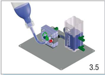
8. Attach the water bottle to the bottom connector on the oxygen side of the RFC with the included tubing (Fig. 3.5).
