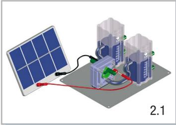
1. Use the cables to connect the solar module to the appropriate terminals on the RFC. When doing so, make sure that the polarity is correct (red = "+", black = "-"). The cell will begin to produce hydrogen and oxygen in a 2:1 ratio (Fig. 2.1).
