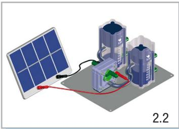
2. Oxygen is produced on the positive side of the cell, and hydrogen on the negative side. The gases collect in the gas storage tanks and displace the water there into the compensation tanks (Fig. 2.2).
