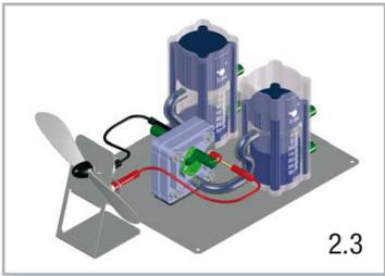
1. When the solar module is unplugged, ensure the motor is switched off, then plug the wires from the chassis into the RFC taking care to use correct polarity (red = "+", black = "-"). When switched on, the cell will use the stored gas to generate current, along with water and small amounts of heat (Fig. 2.3).
